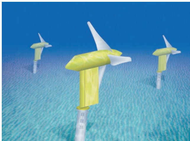
FIGURE 7.29 Power from ocean currents. A prototype of an ocean current power system, which uses a field of underwater turbines anchored to the ocean floor. As currents flow past the turbines, they turn the rotors and generate electricity. The turbines can swivel on their anchors to face oncoming currents, so this system is also useful in locations where strong tidal flows occur.
