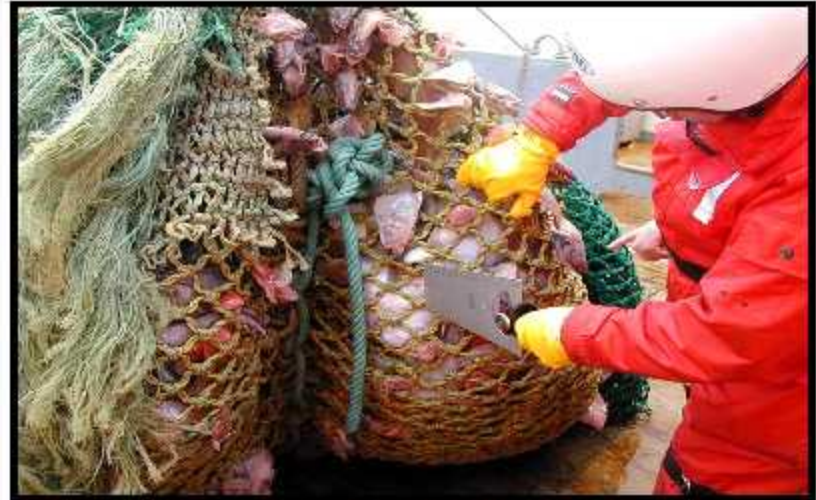
Measuring the recovered net using a gauge. Juvenile fish cannot escape through the small (illegal) mesh.
